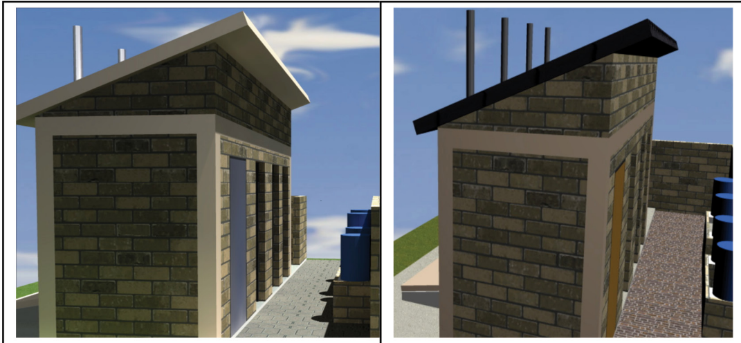
Fig 5.13 Latrines for boys (right) and girls showing hand-washing stands
